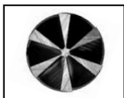
Bottom surface of 6HFSS cutting edge
