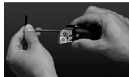
3. Tighten 3 bolts to attach the head
