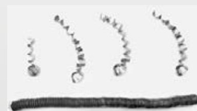
Chips by SM chipbreaker (SUS304)
